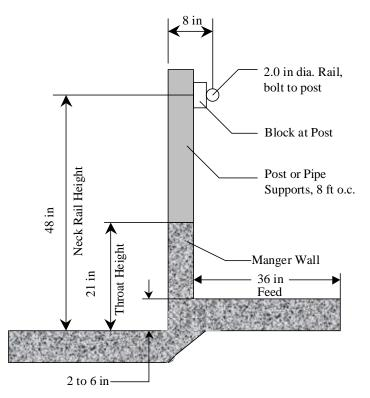
**Figure 2.** Post and rail feeding fence for cows (adapted from Graves, 1998).
