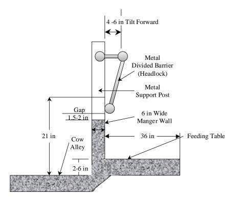
**Figure 3.** Divided feed barrier (headlock) (adapted from Graves, 1998).
